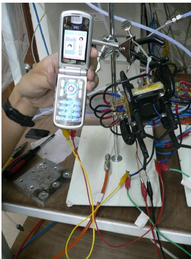
Fig. 14. The demonstration of the 10-cell air-breathing miniature PEMFC powered cell phone directly without converters/inverters.
